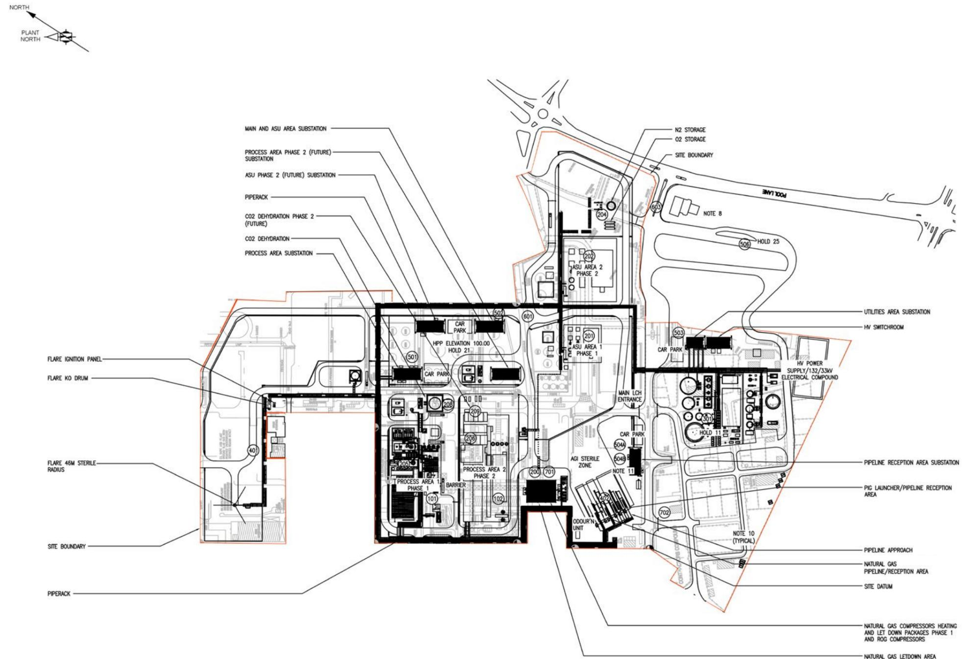
Figure 8.2<sup>22</sup> - HyNet Hydrogen Production Plants 1 and 2 Plot Plan.
